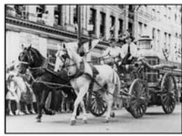
The city's second steam fire engine was a third-rate 1903 American LaFrance Metropolitan with a 600 GPM capacity. Delivered on July 7, 1903, it had a wooden frame and a wooden pump house. It was operated by the newly formed L.A. Muller Steamer Company until 1912. The steamer is pictured on May 21, 1940, at a transportation parade on Franklin Street.
